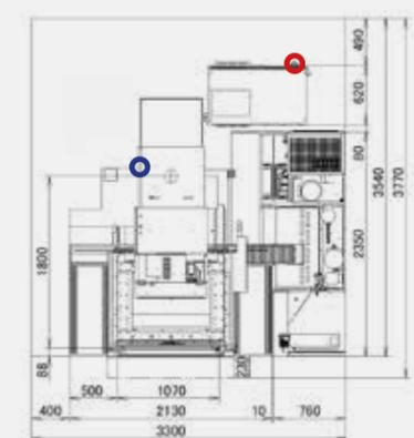
\*] The above floor plan is that of a standard type machine. Contact FANUC if you wish to order options such as Z axis travel 410 mm, 510 mm and 30 kg wire loader options.
