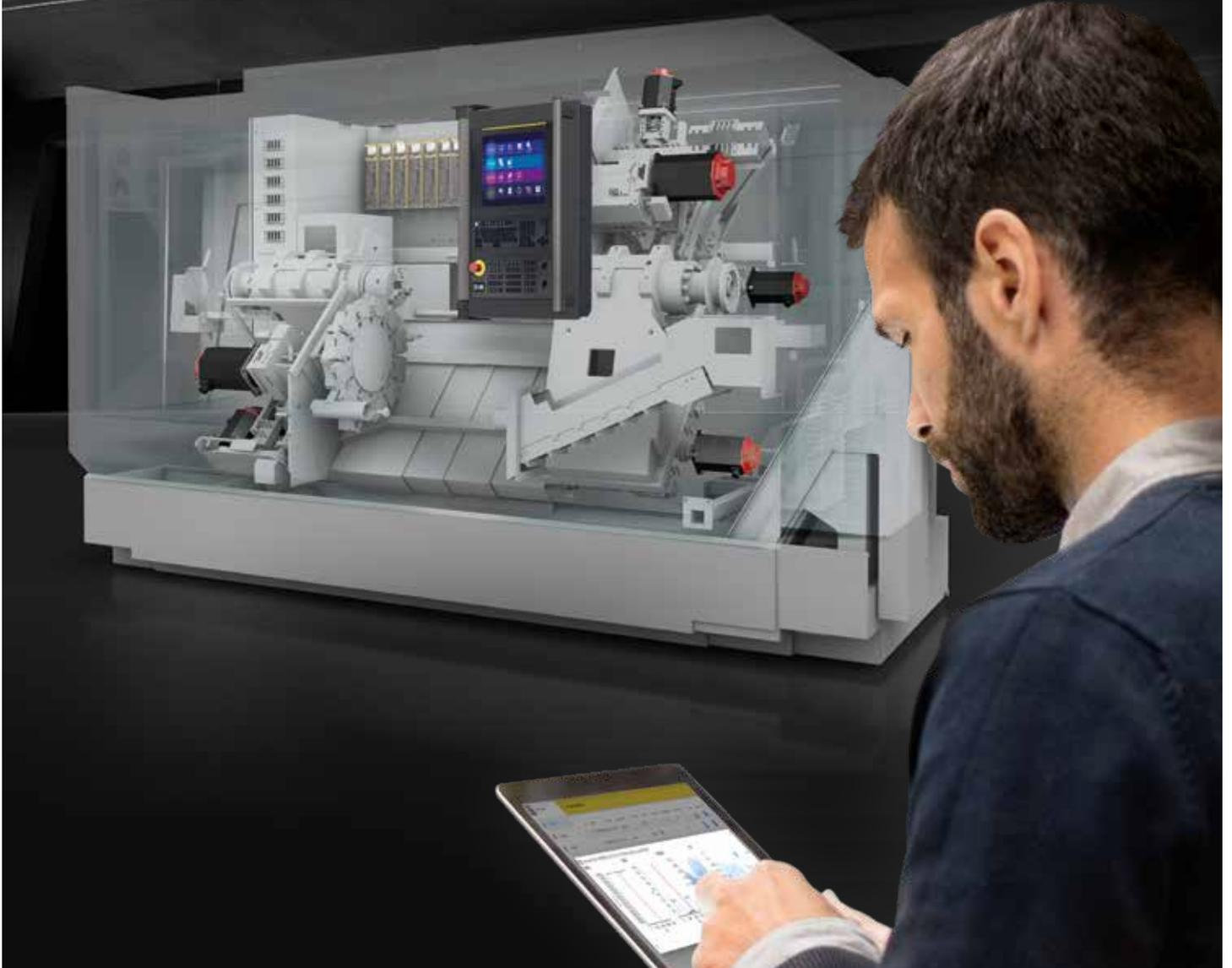
AI Servo Monitor is a software that visualises anomalies of drive systems for servos and spindles through machine learning. It can analyse daily processing data and display the results in intuitive graphs.
