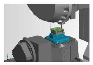
FANUC CNC Reflection Studio is a Windows® application that simplifies CNC part program creation and editing, offering immersive CNC machine animation for visualising machine behaviour, workpieces, fixtures, and tooling setups.
