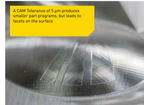
A CAM Tolerance of 5 µm produces smaller part programs, but leads to facets on the surface
