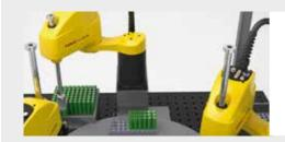
FANUC SCARA robots are ideally suited to robotic assembly, robotic pick and place, inspection and robotic packaging applications.
