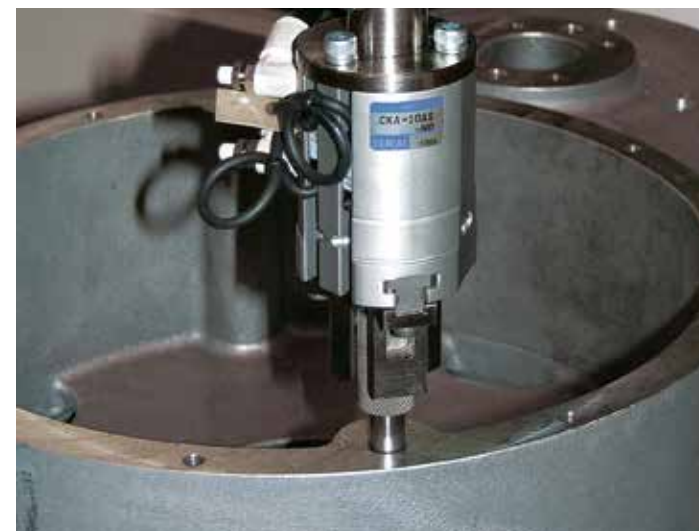
Dimension check of holes (Gage insertion by force control)
