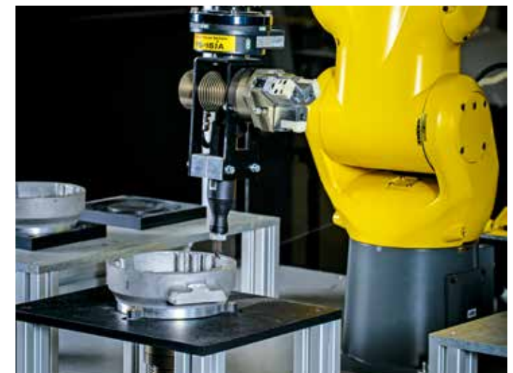
Force controlled deburring
