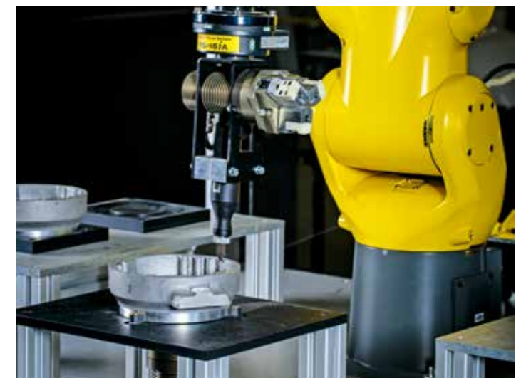
Force controlled deburring
