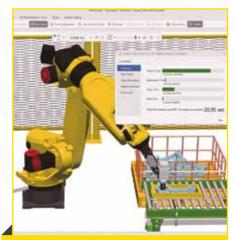
Pre-program robots by starting programming before installation, confirming trajectories, and validating DCS zones before downloading them to the real robot.
